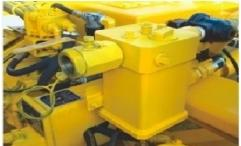
**Lubricator**: Lubricator provides drilling system( hammer & drill pipe), regular maintenance of the lubricator with dedicated lubricating Oil will improve the drilling efficiency and service life.
