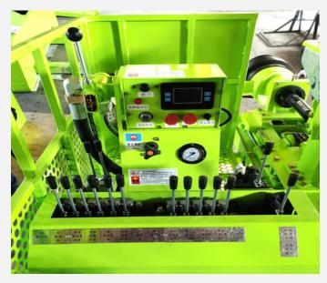
New integrated operation console, digital display engine instrument, real-time monitoring of engine running status, advanced hydraulic system, make operation safer and more convenient
