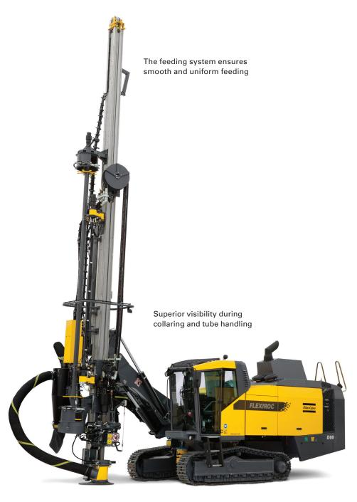
The safety cabin is ROPS and FOPS approved mounted on a protective plate.
