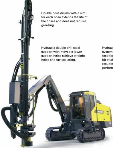
Hydraulic cylinder-feeding system ensures that the adjusted feed force is applied to the drill bit at all times during drilling, resulting in improved rock tool performance and productivity.
