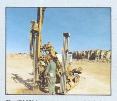
The CM-351 is a compact, powerful rig for drifter or downhole drilling of  $64\text{-}140\text{-}\mathrm{mm}$  ( $2\frac{1}{2}$  to  $5\frac{1}{2}$ ") blastholes. Fixed-length boom. Its 2.2-m ( $7\frac{3}{3}$ ") width makes it easy to transport.
