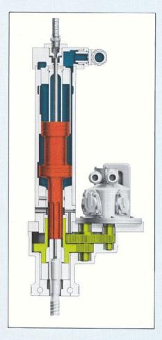
The EVL-130 drifter is easy to service in the field, if required. To remove the shankpiece, just snap out a split ring and push out two pins. The internals can easily be changed by one man in a few minutes.
