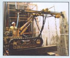
The LM-100 is ideal for small jobs in confined places; it makes fast work of holes 44-64 mm ( $1\frac{3}{4}$  to  $2\frac{1}{2}$ "). Compact, but uses a 3-m (10-ft.) rod change.
