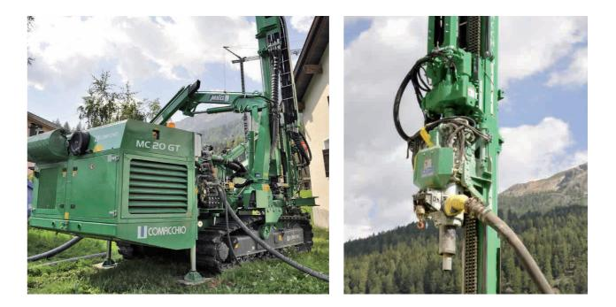
High-performance hydraulic drilling rig with double head system able to fulfil:
