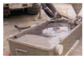
In both cases the drill cuttings are conveyed and collected through special systems in order to avoid the pollution of the environment in which the drilling is performed.
