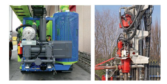
Unique in the world and exceptional in many ways, the GEO 909 GT was awarded a Special mention for Technical Innovation at the International SAMOTER show in 2008. Its design is based on the main features of the GEO 900 GT, but it's distinguished by a PATENTED automatic loading system for both drilling rods and casings with 122 meters capacity (400 ft) that allows one single driller to operate the machine, thus reducing operating costs and improving safety. The machine can perform:
