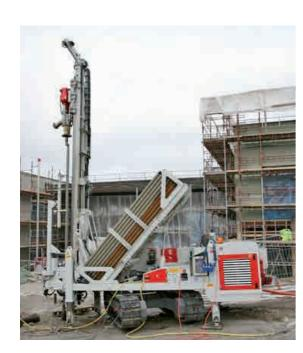
GEO 655 with automatic pipe handling system
