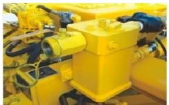
**Lubricator**: Lubricator provides drilling system( hammer & drill pipe), regular maintenance of the lubricator with dedicated lubricating Oil will improve the drilling efficiency and service life.
