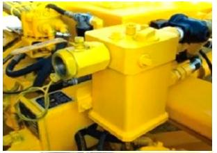
**Lubricator**: Lubricator provides drilling system( hammer & drill pipe), and various air motor lubrication, regular maintenance of the lubricator with dedicated lubricating Oil will improve the drilling efficiency and service life.
