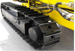
**Traveling System**: each crawler were all powered by air motor, driven by a closed-end reducing gear, brake through the spring brake system, air clutch, same power of positive and negative direction, the gradeability arrives 35° while drag a compressor.
