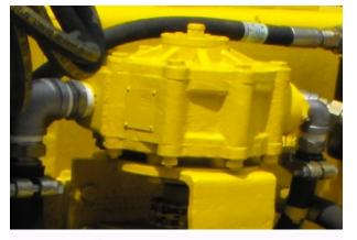
**Hydraulic Pump Station:** Vane Air Motors and hydraulic pump are core parts of hydraulic Pump Station, which provide sufficient driving force to the hydraulic cylinder to ensure the accurate orientation capability of boom assembly.
