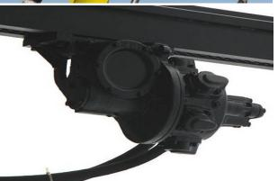
Rotary Head Assembly: The Rotary Head Assembly speed reduced by two planetary gear, the output torque is 2150N/m, rotary speed 0-72rp/m, Rotary with impact cushioning capacity, with the ability to reduce the impact of drilling reaction forces transmitted to the rotary motor, to reduce parts wastage, simple internal structure, easy maintenance. rotary motor equipped YX ring, and thrust needle roller bearings equipped U.S. IR OEM product, increase the capability and life.
