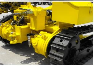
**Crawler**: each side of frame equipped an oscillating cylinder, hick powered the crawler can up-down floating in the range of 15 degrees, which ensure the keep balance while the drill is walking and working, advanced plate designing make the crawler have high grip capability.
