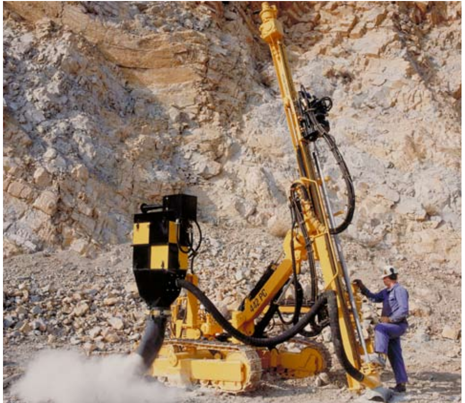
ROC 442PC with dust collector and front mounted control panel.
