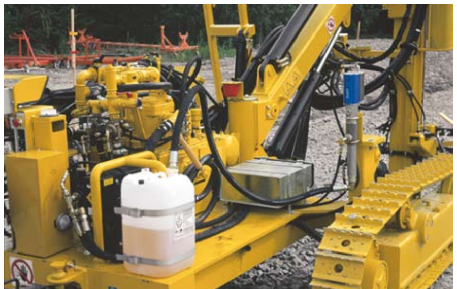
Foam flushing system (optional)
