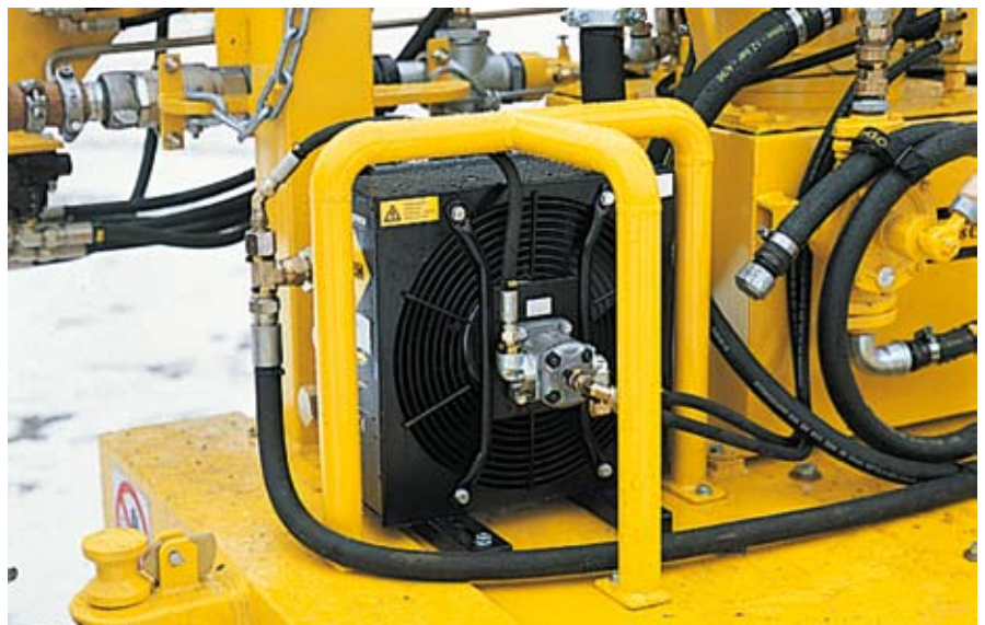
ROC 442PC is equipped with oil cooler as standard
