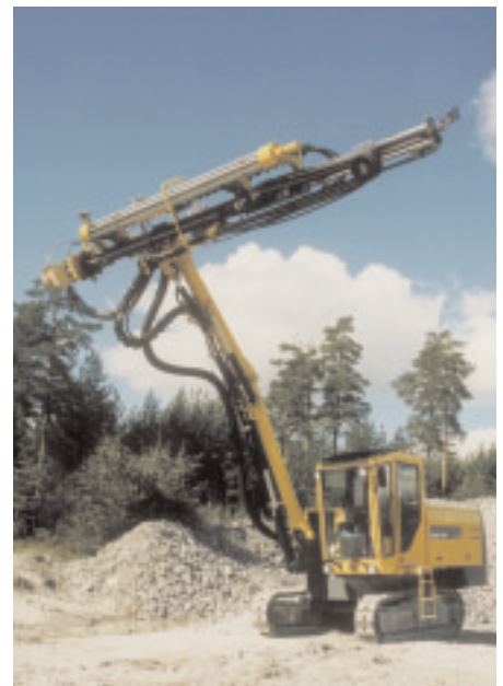
The versatile boom head allows for, easy service access of the rock drill and horizontal drilling.
