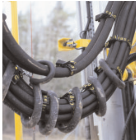
The separated hydraulic percussion hoses system means less wear and easy service.
