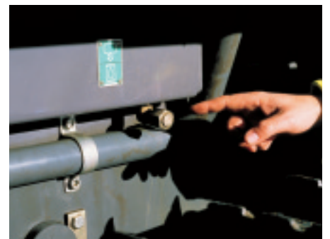
Oil-drainage points are easily accessible. Atlas Copco recommends bio-degradable hydraulic oil.
