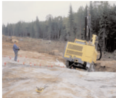
The optional hydraulic winch can be used to anchor the rig in extreme conditions.
