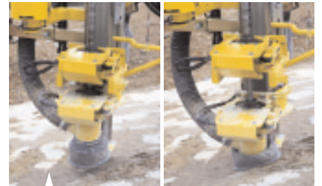
Double drill steel supports gives better collaring and straighter holes.
