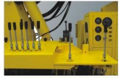
**Operating System:** Operating System equipped in the back of rig, easy drill operator o observe and centralized control the machinery and hydraulic system, the pneumatic operating system is convenient and safety, could be one-handed control while traveling.
