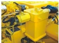
**Lubricator**: Lubricator provides drilling system( hammer & drill pipe), regular maintenance of the lubricator with dedicated lubricating Oil will improve the drilling efficiency and service life.
