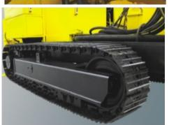
**Traveling System:** Each crawler were all powered by imported high power hydraulic motor, driven by a closed-end reducing gear, brake through the spring brake system, air clutch, same power of positive and negative direction, the gradeability arrives 35° while drag a compressor.
