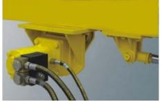
**Drill Guide Assembly:**Drill Guide Assembly:Heavy structure drill guide with Manganese steel rail trim & Multiple roller designing ,make the guide can withstand high torque, resistance to deformation,also can greatly extend the life of skateboarding and guide,and effectually guarantee the various drilling angle.
